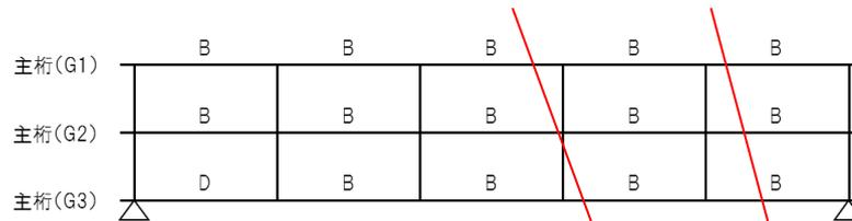
$$\text{損傷評価点 [DG]} = 0.67 \times (25 \times 0.9 + 75 \times 0.1) = 20.1$$
